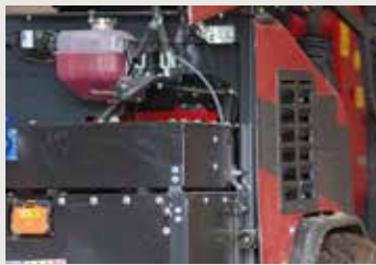
Motors are water cooled, with a radiator to the right of the user.
