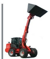
Development of the first telescopic wheel loader with articulated joint, the 870 T.
