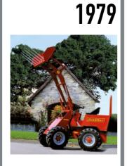
Development of the first D25 compact wheel loader (28 hp), a crucial moment in the company's history. It is the first loader with hydrostatic drive and quick-change system on the global market.
